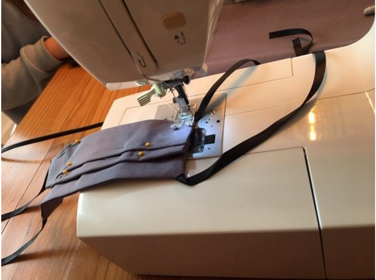
Step 15 : Complete sewing on both shorter 7" sides of the mask to permanently secure the pleats.
